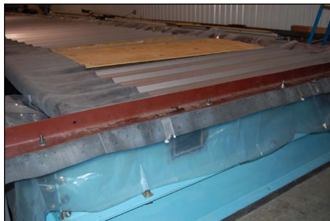
Figure 3.12. Sixty Mil EPDM Lining and Angle Connections
